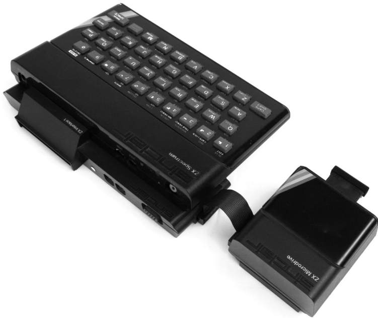
Fig 1.9 The Microdrive plugged into the Interface 1, which sat beneath the Spectrum. Up to eight in a row could be connected.
